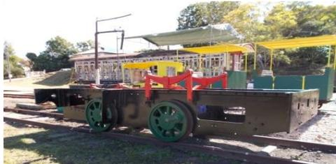
The frame is now mounted on the axles and wheels after a somewhat steep learning curve. The way to do it was NOT to try and lift the wheels, axles and axle boxes into the frame, but to lower the frame onto each pair of axle boxes one at a time.
